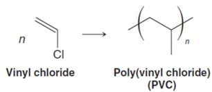
The little "n" indicates that there are a bunch of vinyl chloride molecules (which are monomers) connected together in order to make the larger polymer, polyvinyl chloride (PVC).
