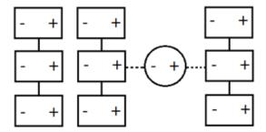
The circle represents the plasticizer molecule, and the rectangles represent PVC molecules. The pluses and minuses represent electrostatic charges, which attract and repel each other. The plasticizer molecule interferes between the strong electrostatic forces between the individual PVC molecules, which means that the PVC molecules are less packed together. As a result, the overall PVC material is more flexible!
